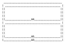
The split-window call has created a new live window, denoted by W5. It has also created a new internal window, denoted by W3, which becomes the root window and the parent of both W4 and W5.
